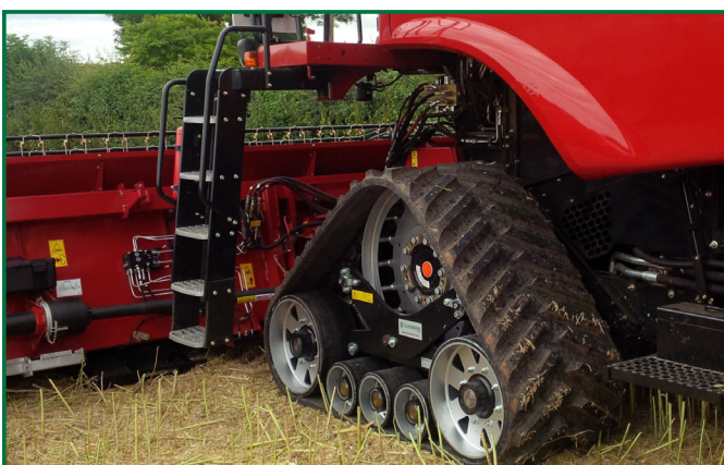
Up to 3x less ground pressure compared to tires with comparable width
