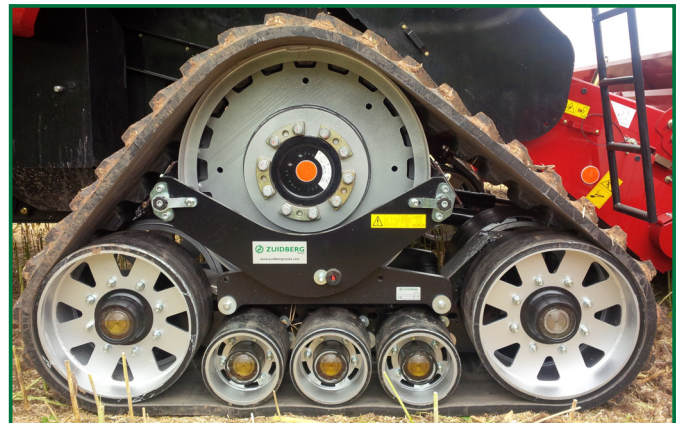
Bogie System (increases driving comfort and improves the ground contour)
