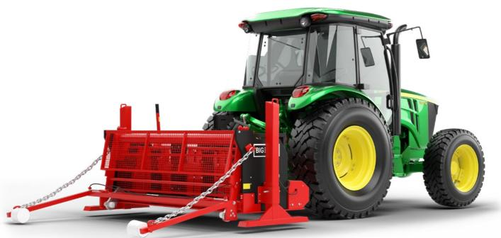
The BigTick® 1040 is durable, heavyweight, and features a solid design. It is the best, most economical solution for harvesting high-quality large turf rolls. The operation speed offered by BigTick enables a high production capacity. The turf rolls have a maximum width of 40 inches (1 m). With a center colter disk installed, the option of harvesting two 20 inch (0.5 m) rolls is also available.
