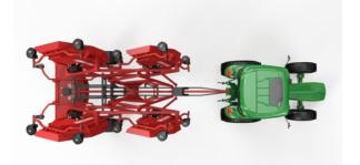
The MowTick® R5582 is an easy to maintain mower with five cutting decks, each with five blades. The MowTick® R5582 can be controlled from the tractor and in the transporting position the MowTick® Rotary not only folds upwards but backwards as well. This results in a low transporting height making it easy to move around.
