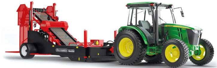
The BigSlab® 3040 is specially designed for harvesting turf for medium to large projects, such as parks and soccer fields. Ideal to market your high-quality turf. With the BigSlab® 3040, you will enjoy impressive speed, efficiency in cutting, and easy transport and placement of the turf with minimum effort.
