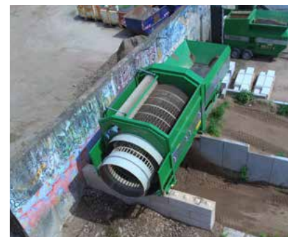
MS 4200-ST Consisting of a feed hopper and double drum
