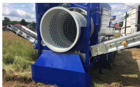
SPECIAL PAINT AND DEFLECTOR PLATE 3. FRACTION
