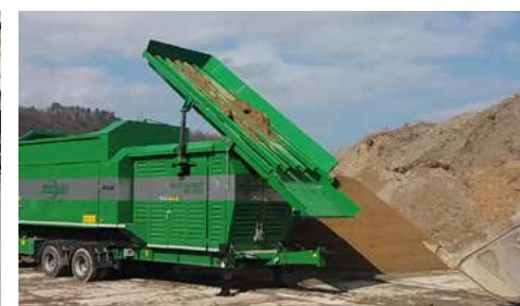
HYDRAULICALLY FOLDABLE STONE GRID (possibility of 4th fraction)
