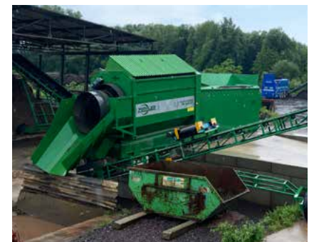
MS 5200-ST with 7 metre long feed hopper and staircase unit.
