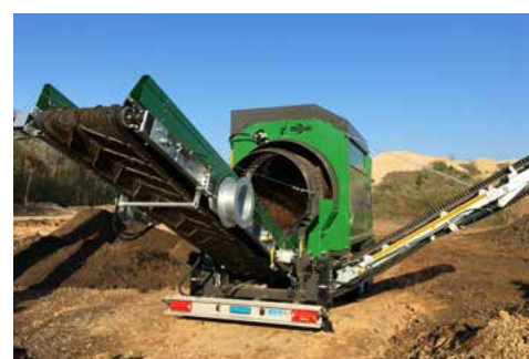
EXTENDED BELTS AND WEATHER PROTECTION ROOF
